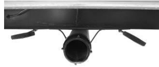
Black/Grey tank drain & valves
