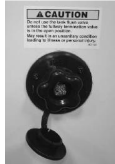
Tank Flush Inlet
