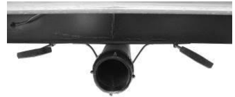
Black/Grey Tank Drain and Valves
