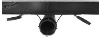
Black/Grey Tank Drain and Valves
