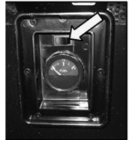
Master / Emergency Shutoff and Fuel Gauge
