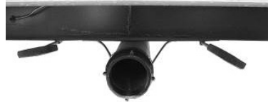
Black/Grey Tank Drain and Valves
