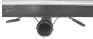
Black/Grey Tank Drain and Valves
