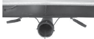
Black/Grey Tank Drain and Valves
