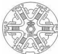
7-way trailer plug car end, rear view
