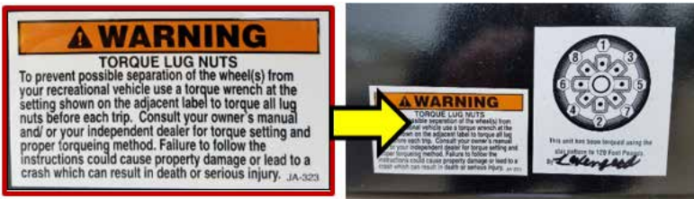
Lug nut torque pattern and warning label
