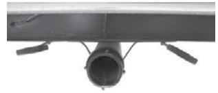
Black/Grey Tank Drain and Valves
