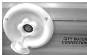
City Water Fill with City Water Connection label the
