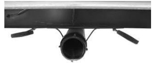
Black/Grey tank drain & valves
